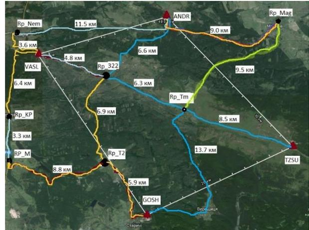
Fig. 2. Scheme of geometric leveling net of II class
