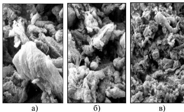
Pic.2. Soil sample microstructure a, b, c); secondary electronic emission mode; Mkrat= 1000, 500, 250
