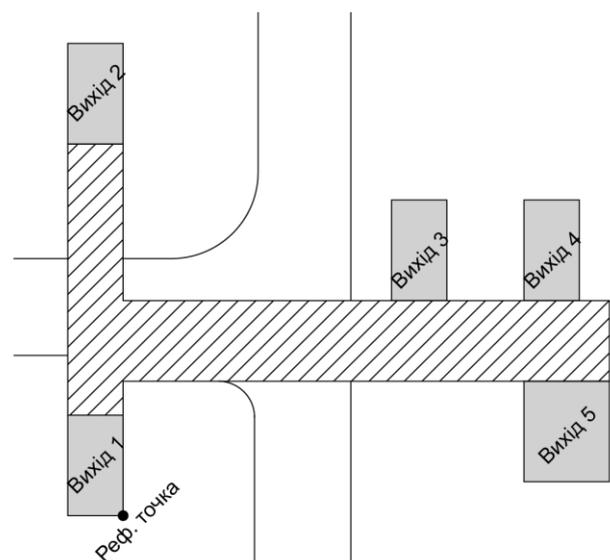
Fig. 2. Underground crossing scheme (Underground and above-ground parts)
