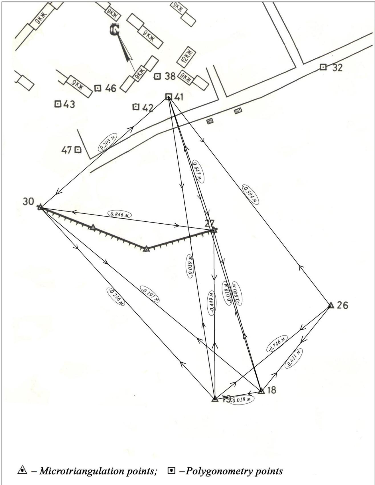
Fig. 3. Directions and distances between the change in the network on the section " Sokol " (Spring 2015)
