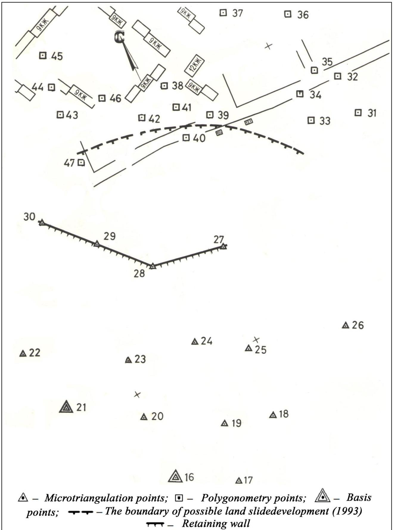
Fig. 1. Scheme of points tracking station on the section " Sokol " (Autumn 1993)
