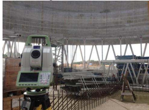
Fig. 8 Cooling tower monitoring using multistation
