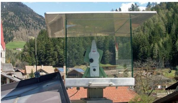
*Fig. 4 Mountainous area monitoring using total station*
