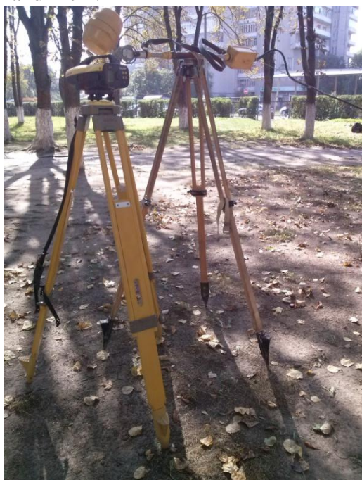
Pic. 1 Installing digital magnetometer and leveling the base point
